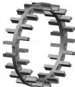
Fig. 49. One-piece finger-type cage.
