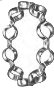
Fig. 52. Pressed-steel welded cage.
