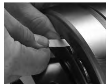
Fig. 95. Measure of RIC before installation.
