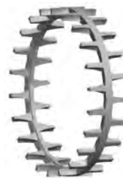
Fig. 44. One-piece, machined-brass, roller-riding, finger-type cage.
