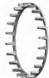
Fig. 46. Split, machined-brass, land-riding, finger-type cage.
