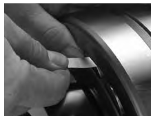
Fig. 91. Measure RIC before installation.
