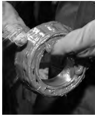
Fig. 147. Grease can easily be packed by hand.
