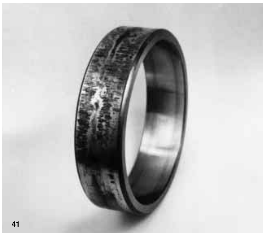
Fig 41 Smeared outside surface of a spherical roller bearing outer ring. Material transfer has occurred from housing bore to bearing ring
