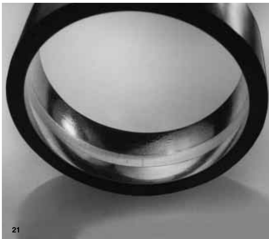
Fig 20 Cylindrical roller with mirror-like surface on account of lubricant starvation
