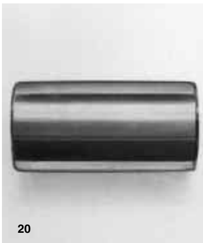
Fig 20 Cylindrical roller with mirror-like surface on account of lubricant starvation
