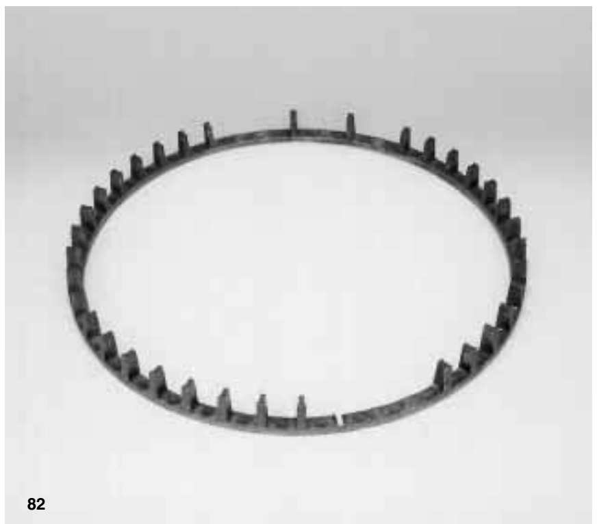
Fig 82 Cage of a spherical roller bearing. Fatigue cracks have formed in the fillets
