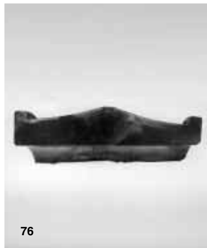
Fig 76 Fractured surface of the inner ring in fig 75
