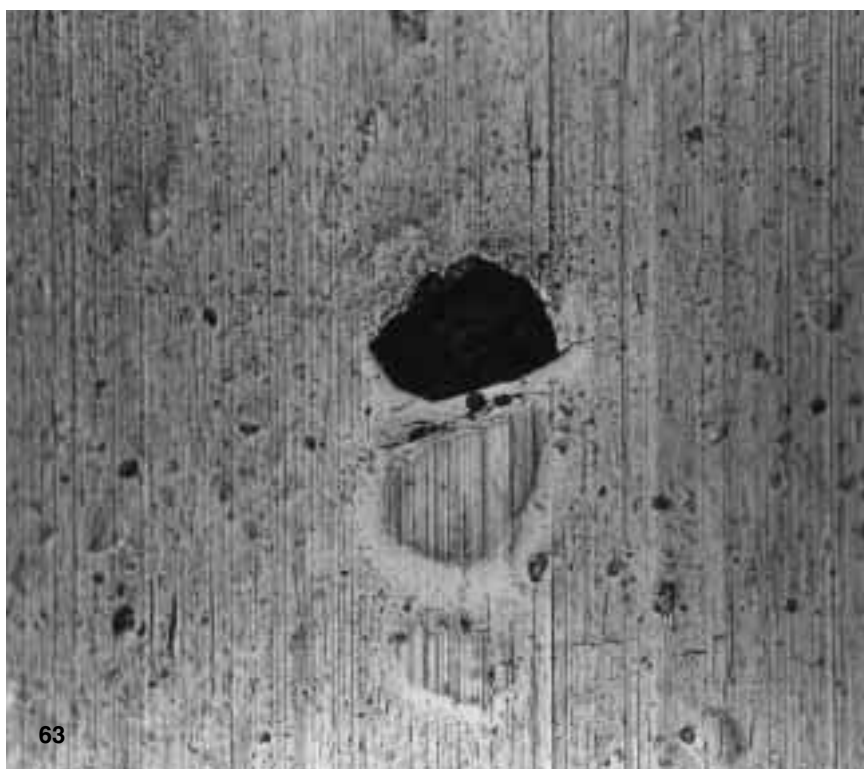
Fig 62 Various stages of flaking in the inner ring of a deep groove ball bearing. The ring has been mounted with interference fit on the shaft and blows have been directed against the outer ring, causing the mounting force to pass through the balls, which have produced the indentations
