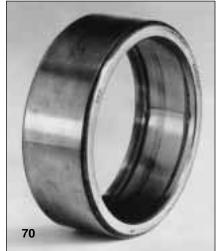
Fig 70 The outer ring of a self-aligning ball bearing with flaking caused by craters that have formed in conjunction with the passage of electric current. It is evident that the flaking has originated at the craters, from where it has spread out in both directions. Detached fragments of flaked material have in turn caused indentations and further flaking
